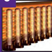
**Re-heat station by infra red heating lamps**
